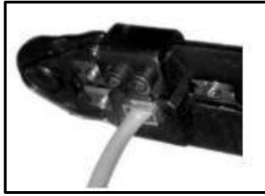
Fig.No.5.9. Crimping the Cable
